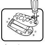
4. Replace the battery cover and tighten the screw to secure the battery cover.
